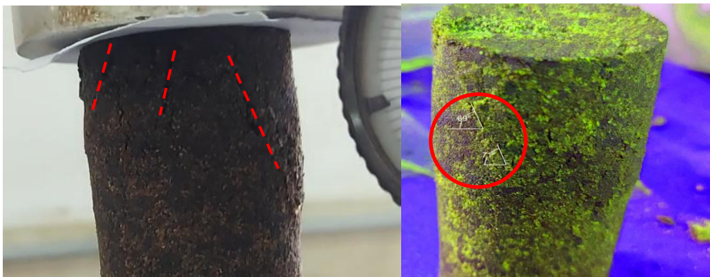
Figure 7: The propagation of cracks in the sample post-failure
