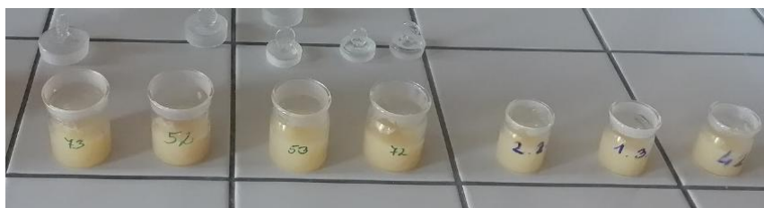
Figure 1: The prepared gelatin gels, from left to right: 7th experiment third fraction, 5th experiment second fraction, 5th experiment third fraction, 7th experiment second fraction, 2nd experiment second fraction, 1st experiment third fraction, and 4th experiment second fraction. 13
